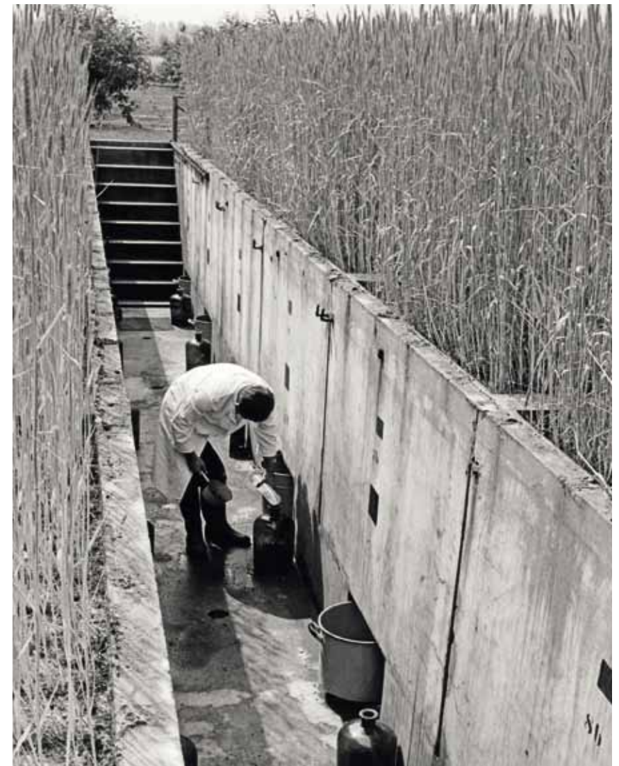
In the lysimeter plant, leachate was collected in vessels and then analyzed
